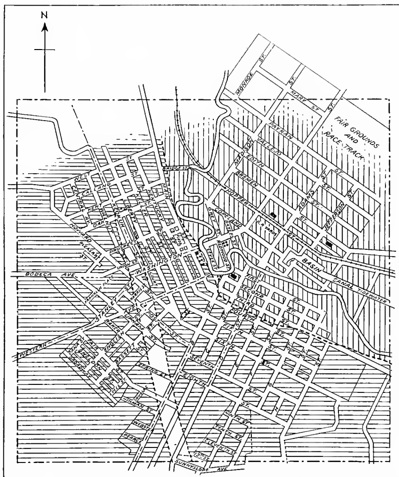
FIG. 64. — Distribution of intensity in Petaluma. Vertical lines represent area of low alluvial land, on which nearly all chimneys were damaged. Horizontal lines represent slopes underlain by rock, on which about half the chimneys were damaged. The solid black areas and dots represent exceptionally severe damage. The blank area inclosed by dotted lines represents a belt of practically no damage. By R. S. Holway.
